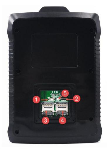
**1 Power switch**: Turn the switch to the left, power on the device; Turn the switch to the right, power off the device.
